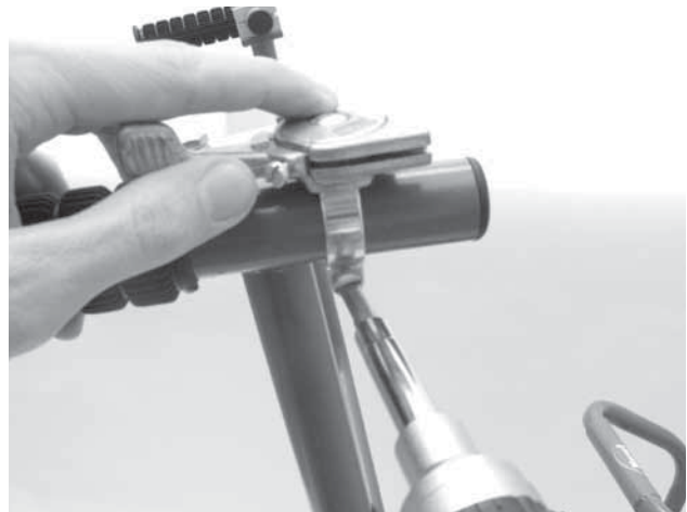
Step 4 – Attach the throttle lever to the "T" grip handle, as shown above.
