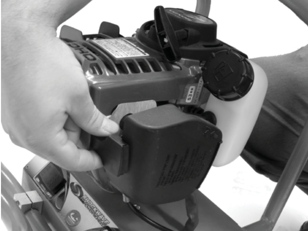
Step 1 – Remove carburetor cover by pressing clips.
